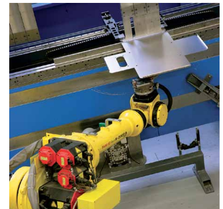
Our bending cell used for making sheet steel enclosures offers flexible dimensioning without tool changes.
