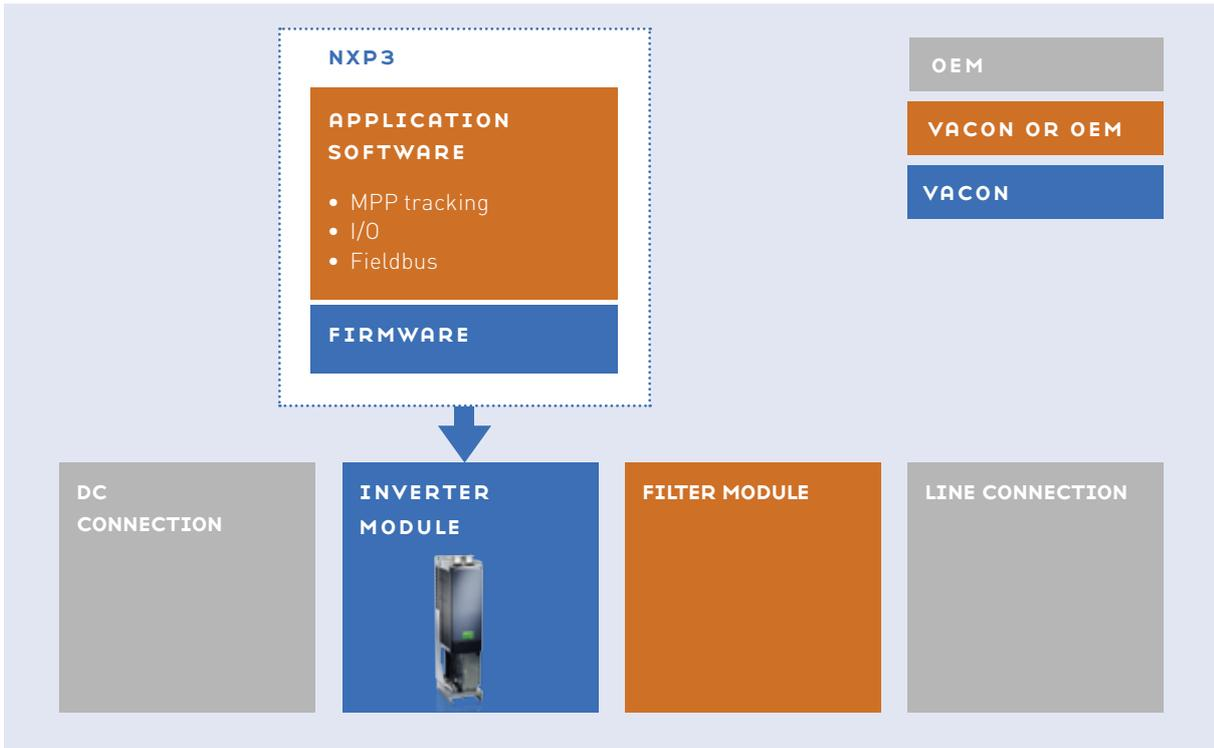
Topology example of a PV inverter system for photovoltaic systems based on Vacon modules for solar inverters. Customers have an option to build their own application software and select the filter, although Vacon can offer both for maximum performance and optimization. Engineering support for solution tailoring is also available.
